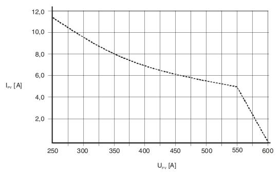
Fig. 4.2: Maximum Input Current of the Sunny Boy 2500U
