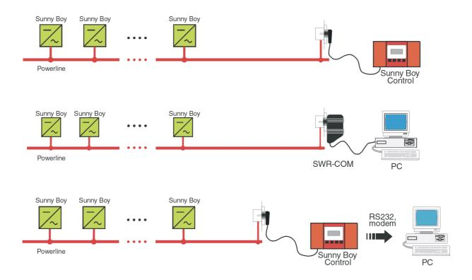
Fig. 3.1: Example of data transmission via Powerline
