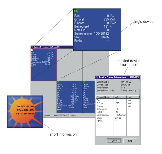
Fig. 3.5: Sunny Data Control user interface
