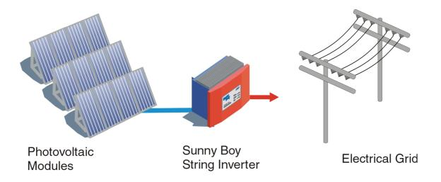
Fig. 2.1: Grid tied string inverter application
