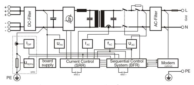
Fig. 2.2: Block circuit diagram of the Sunny Boy 2500U
